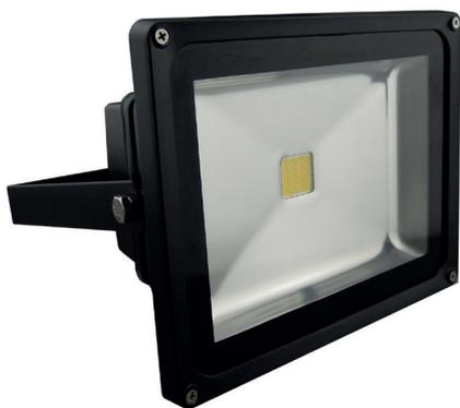
BAI LED Floodlight HQ 30W 6500K 3000lm 100-240V DC IP65 IK08 Alu housing black 120D 2m cable
