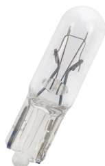
WB20240401 T5 Wedge 24V 40mA 1W 10000h C-2F
