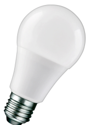
145630 LED Industry A60 E27 9.5W (83W) 1200lm 840 100V-260V AC/DC
